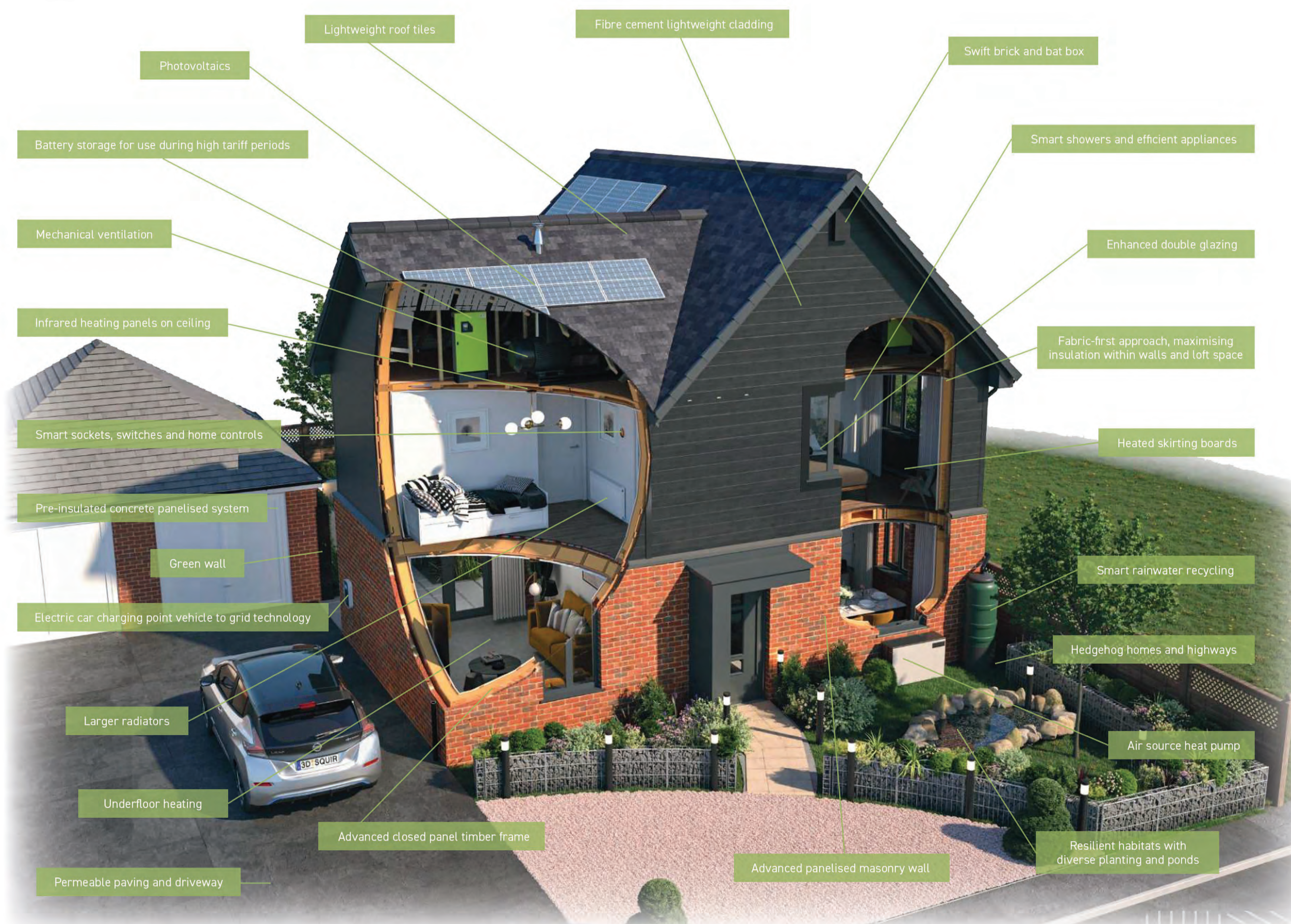
The Zed House – The first zero carbon house by a major housebuilder to substantially surpass the Future Homes Standard, delivering over 125% improvement in carbon emissions
